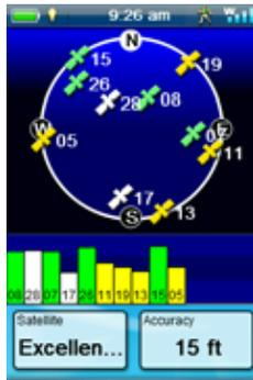
The Satellite Status screen displays a graphical representation of the satellites overhead in relation to your current location (the center of the circle). The color of the satellite graphics, as well as the bar graph, indicate the signal strength of the signals being received. The numbers indicate the assigned satellite designation. The data fields at the bottom of the display are customizable (see *Customizing the Data Fields*).
